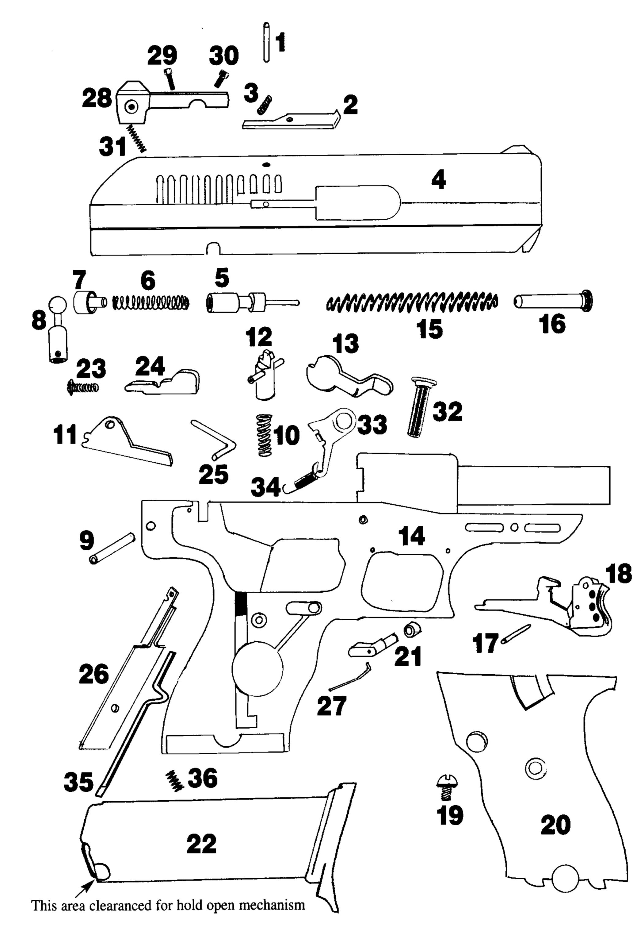
ATTENTION: This pistol is equipped with a last round hold open mechanism. Older Hi-Point magazines may not have the proper clearance for this mechanism. Unclearanced magazines WILL DAMAGE the frame if forced into the pistol.
